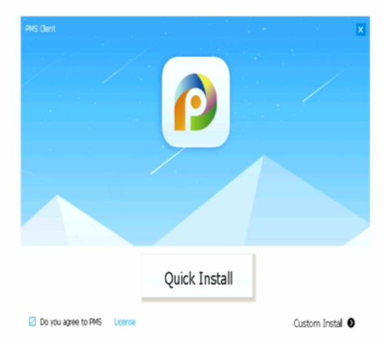
Step 12 Click Quick Install to start installation, or click Custom Install to set the installation path. The installation progress interface is displayed.
