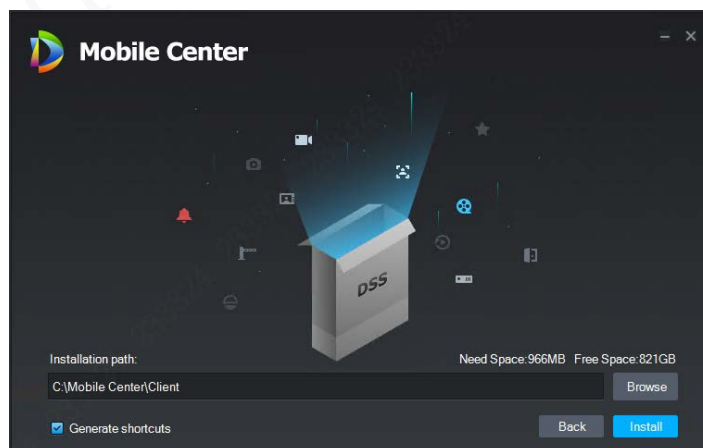
Figure 4-2 Select the installation directory
